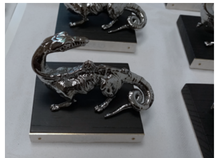
Ruthenium-finish salamander showing all the details reproduced from the 3D model.
