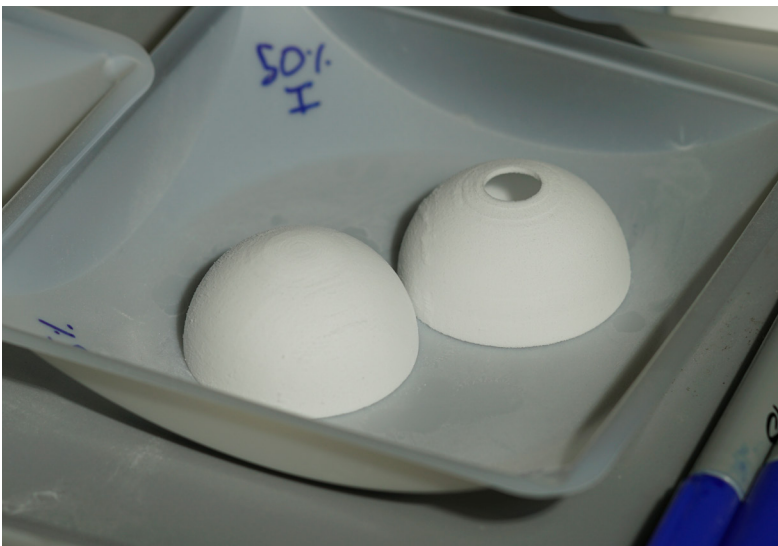
— Fully fired Canopy proprietary reusable TPS formulation in representative shapes, showcasing overhang angles that are achievable with binder jet 3D printing.
