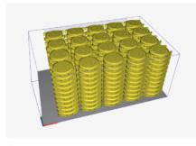
200 watch cases can be printed in a single build cycle on the Desktop Metal Shop System. No support structures are required.
