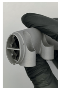
— 3D printed parts for rear dropouts prior to assembly
