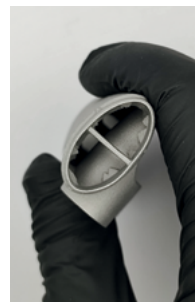
— 3D printed parts for rear dropouts prior to assembly
