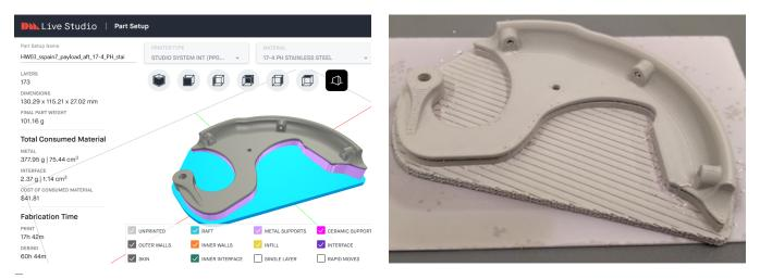
A software-guided workflow navigates users through the metal 3D printing process, from printing to sintering with step-by-step instructions.
