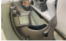
The freedom of design that comes with building a metal part layer-by-layer allowed the team to include complex design features into the hinges with ease.
